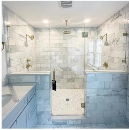
The green tint often seen in glass is caused by iron content used during the manufacturing process. While some find this green hue appealing, others prefer a clearer look. To address this, low-iron glass is available, which significantly reduces the green coloration.
